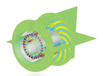
With its unstructured meshing method, elements are automatically adapted allowing for a non-homogenous mesh without any performance degradation.
