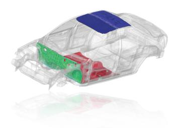
Actran for Nastran provides CAE engineers advanced features for mixing the best of both worlds for trimmed body simulations: an MSC Nastran modal representation of the body and an Actran physical representation for the trim components.
